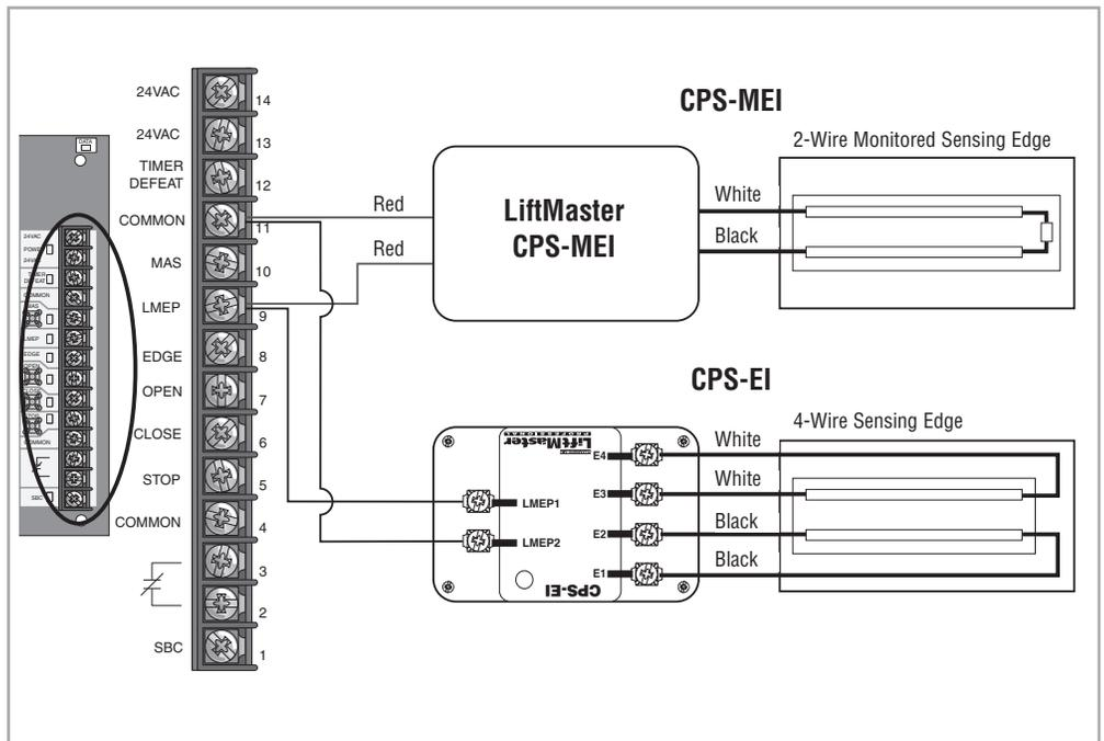
**NOTE:** Only one LMEP device can be connected to the logic board. To attach additional LMEP's, the CPS3CARD option card is required. Secondary (non-monitored) entrapment protection devices (with N.O. dry contact) will be wired to the EDGE and COMMON terminals.
